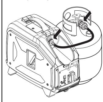
If using a 20 lb. cylinder, open the cylinder valve completely (see page 16).
