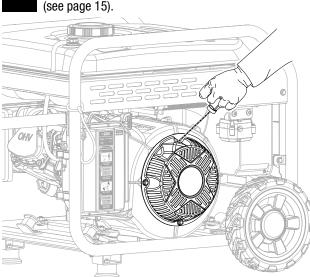
Allow engine to run for 15-30 seconds, then move the choke lever to the RUN position
