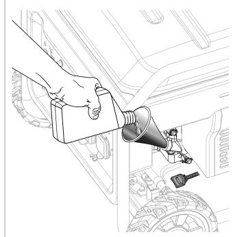
Set unit on flat surface so engine is level. Remove dipstick, wipe clean, put back in hole (but don't screw in) and check lubricant level.
