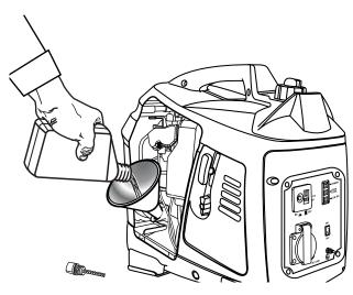
Set unit on flat surface so engine is level. Remove dipstick, wipe clean, put back in hole (but don't screw in) and check lubricant level.
