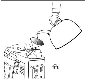
This is a 4-cycle engine. Do not mix fuel and lubricant together.
