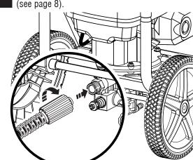
Completely uncoil and straighten high pressure hose to prevent kinks.
