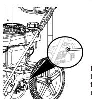
If detergent injection hose comes loose from pressure washer, reattach it here.
