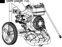
Allow engine to run for several seconds, then move choke lever to RUN position
