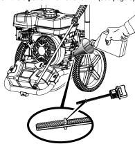
Turn the fuel valve to OFF before adding
