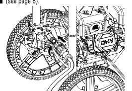
Completely uncoil and straighten high pressure hose to prevent kinks.
