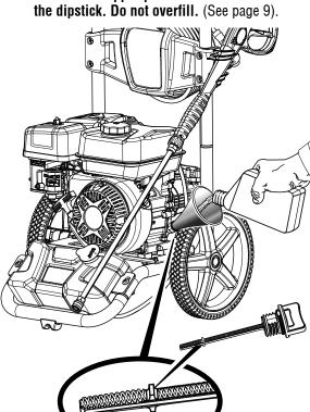
Turn the fuel valve to OFF before adding lubricant.
