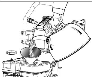
This is a 4-cycle engine. Do not mix fuel and lubricant together.
