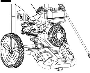
Allow engine to run for several seconds, then move choke lever to RUN position (see page 10).
