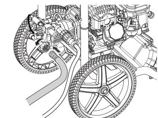
Completely uncoil garden hose or remove completely from reel to prevent kinks.
