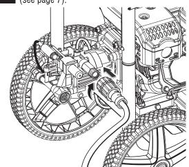
Completely uncoil and straighten high pressure hose to prevent kinks.
