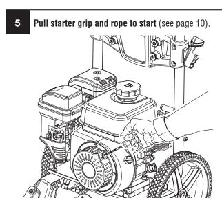
Allow engine to run for several seconds, then move choke lever to RUN position (see page 10).
