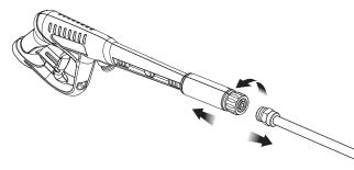
3 Connect the high pressure hose to the trigger
