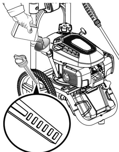
Turn the fuel valve to OFF before adding lubricant.
