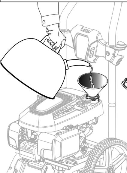
This is a 4-cycle engine. Do not mix fuel and lubricant together.
