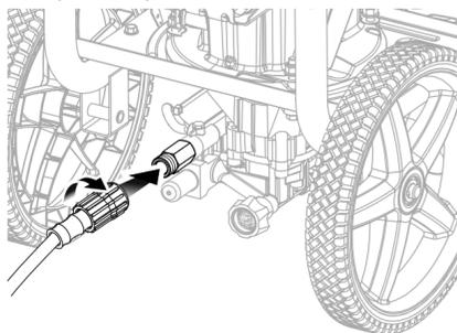
Completely uncoil and straighten high pressure hose to prevent kinks.
