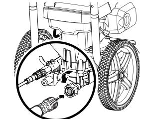
Completely uncoil garden hose or remove completely from reel to prevent kinks.
