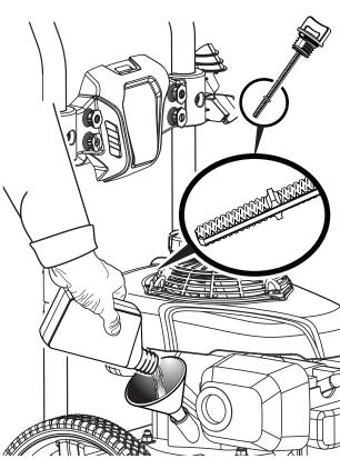
Turn the fuel valve to OFF before adding
