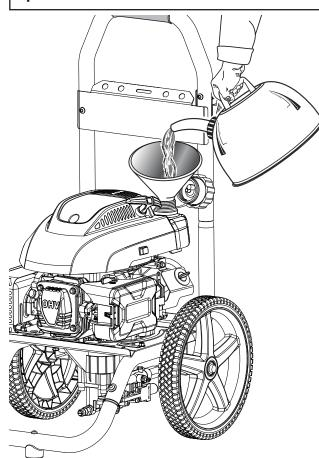
This is a 4-cycle engine. Do not mix fuel and lubricant together.
