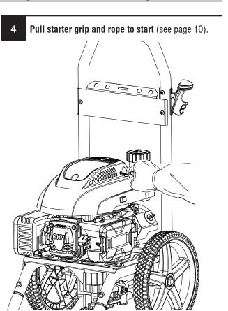
Allow engine to run for several seconds, then move choke to RUN position (see page 10).
