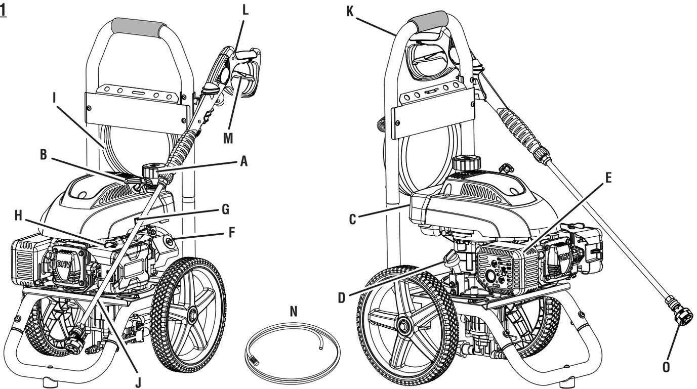
A - Fuel cap (bouchon de carburant, tapa del combustible)
