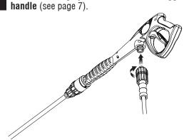
Connect the high pressure hose to the pump
