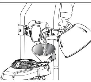
This is a 4-cycle engine. Do not mix fuel and lubricant together.
