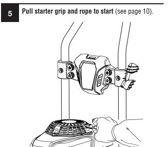
Allow engine to run for several seconds, then move choke to OFF (RUN) position (see page 10).
