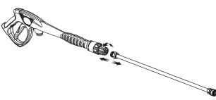
Connect the high pressure hose to the trigger
