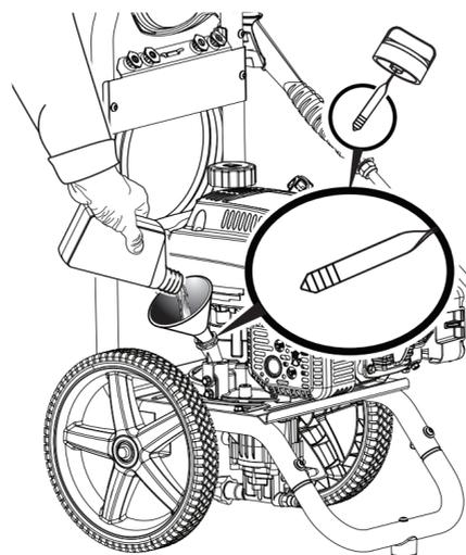
Turn the fuel valve to OFF before adding lubricant.
