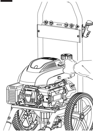
5 Allow engine to run for several seconds, then move choke to OFF (RUN) position (see page 10).
