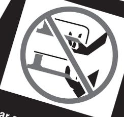
**Risk of injury. Keep hands and feet away from rotating blades. Make sure mower and blades are stopped before placing hands or feet near blades. Do not operate mower unless chute deflector or entire grass catcher is in its proper place. Do not put hands or feet under or into mower when motor is running. Before mowing, clear area of objects that may be thrown by the blade.**
