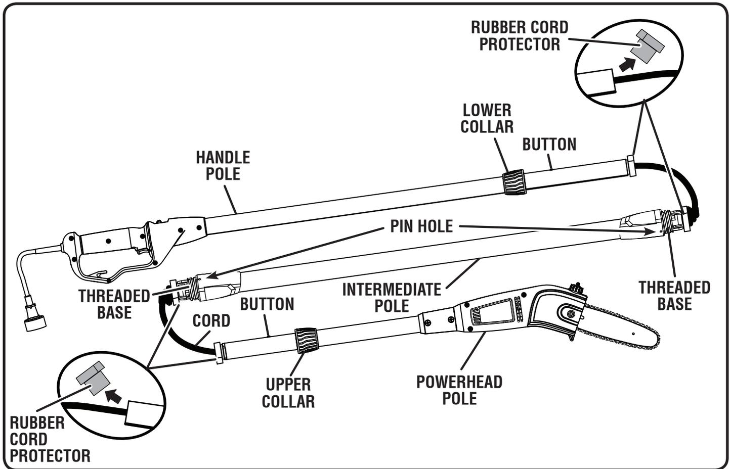
These instructions replace the instructions for **Connecting the Poles** on page 11 of the operator's manual and the figure above replaces figure 3 in the manual artwork.
