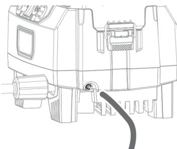
**2** Pour pressure washer detergent into bucket. Connect soap siphon filter to hose and drop in bucket. (see page 11).
