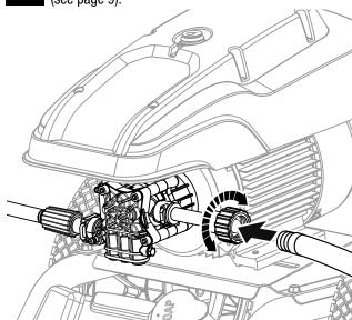
Completely uncoil garden hose or remove completely from reel to prevent kinks.
