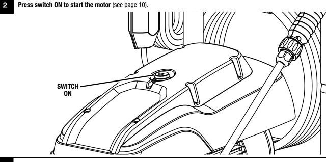
When finished, press switch OFF to stop the motor (see page 10).
