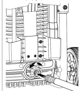
Completely uncoil garden hose or remove completely from reel to prevent kinks.
