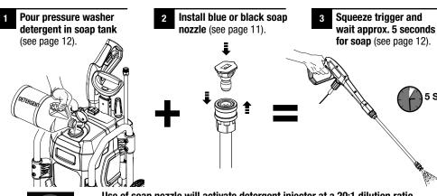
Use of soap nozzle will activate detergent injector at a 20:1 dilution ratio. WARNING! Never use bleach or solvent-based detergent.
