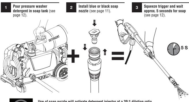
Use of soap nozzle will activate detergent injector at a 20:1 dilution ratio. WARNING! Never use bleach or solvent-based detergent.
