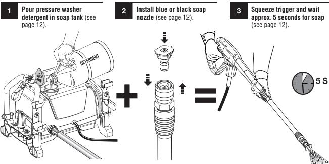
Use of soap nozzle will activate detergent injector at a 20:1 dilution ratio. WARNING! Never use bleach or solvent-based detergent.
