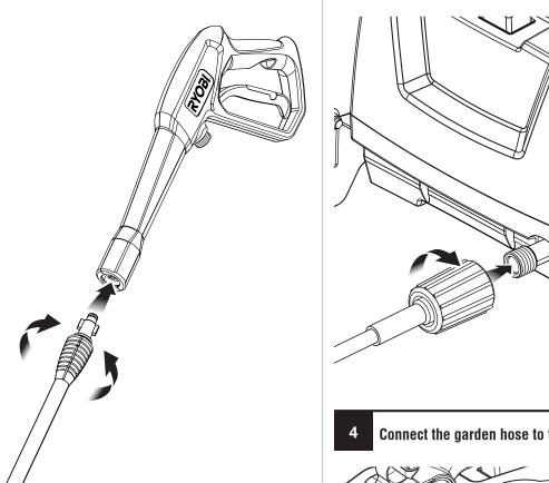
Connect the high pressure hose to the trigger
