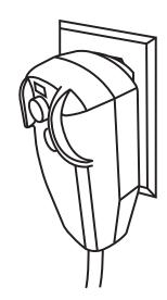
If using an extension cord, arrange a drip loop to avoid the possibility of the tool plug getting wet
