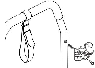
Connect the spray wand to the trigger handle
