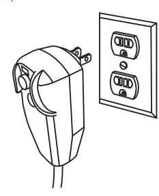
If using an extension cord, arrange a drip loop to avoid the possibility of the tool plug getting wet
