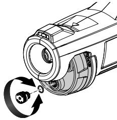
Rotate the nozzle clockwise until the o-ring is sealed against the face of the mode selector. Do not over-tighten.
