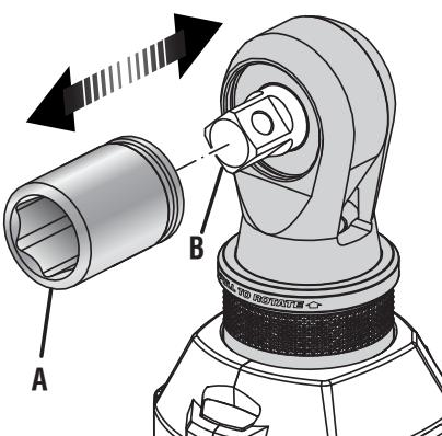
A - 3/8 in. socket (not included)[douille à prise de 9,5 mm (3/8 po) (non inclus), casquillo de 9,5 mm (3/8 pulg.) (no incluida)]
