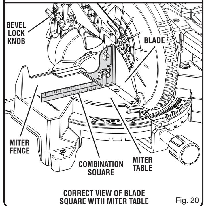
CORRECT VIEW OF BLADE SQUARE WITH MITER TABLE
