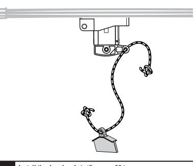
**Install the door bracket.** (See page 26.) NOTE: Installation varies for single panel and wooden garage doors. See page 27 for details.
