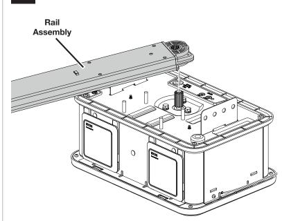
Secure rail assembly to power head. Raise Wi-Fi antenna to upright position. (See page 18.)
