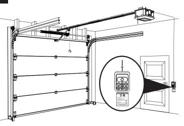
Wire indoor keypad and safety sensors. (See pages 30 - 32.) NOTE: Strip 1/2 in. of insulation from the ends of each wire prior to installation.
