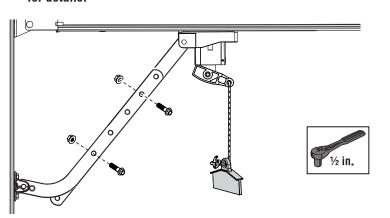
Assemble and install safety sensors. (See page 29.) Align sensors until they are directly facing each other.
