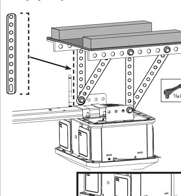
Remove tape and position RF antenna beneath the garage door opener for better signal reception between your opener and the outdoor keypad.
