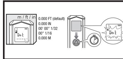
To change the unit of measure, hold the home button for 5 seconds.
