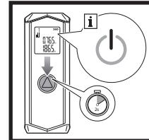
Press the home button for 2 seconds to shut off.
