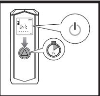
Press the home button for 2 seconds to the last unit measure and shut off.
