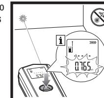
Press the home button to take the measurement. Distance is measured from the back of the unit.
