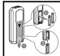
Remove battery cover. Two AAA batteries are pre-installed. Remove pull tab to activate the batteries. Replace cover.
