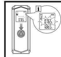
Press home button to lock in measurement. Only the last measurement is saved.
